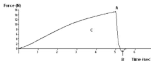
**Fig. 1.** Force-time plot obtained by Texture Analyser [A- Firmness Maximum value of the peak; B-Adhesiveness (Area of negative peak); C-Consistency (area of positive peak)]
