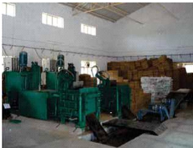
**Fig 1:** Densified Complete Feed Block Making Machine
